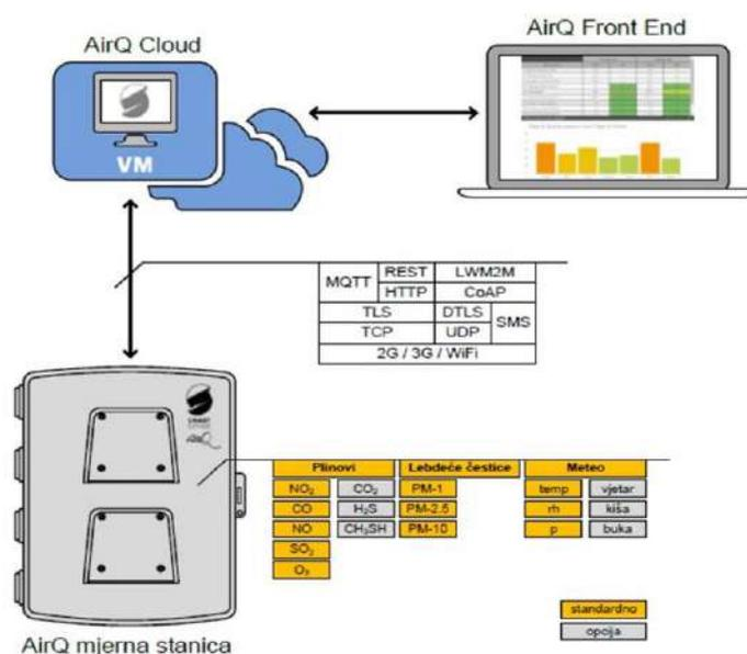
Figure 4 System for monitoring outdoor air quality
